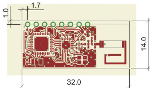
Module Thickness: 2.20 mm +/- 0.20 mm
