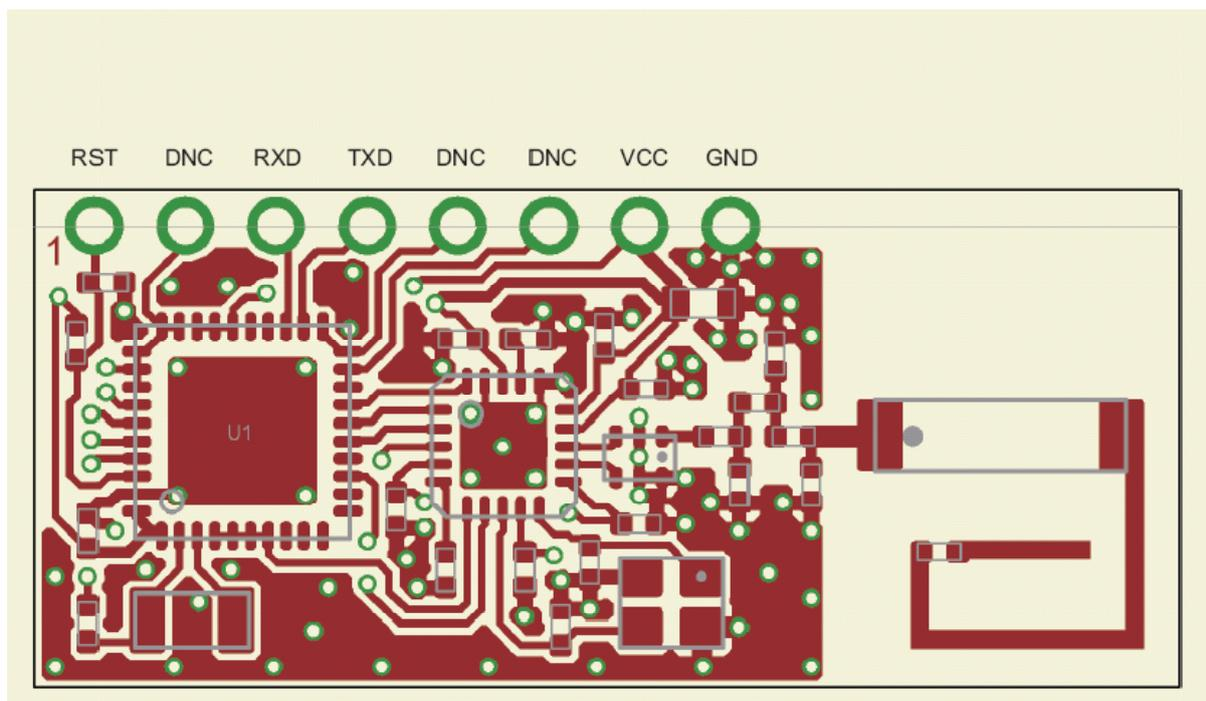
Fig. 1: Receiver module dimensions and connector assignment
